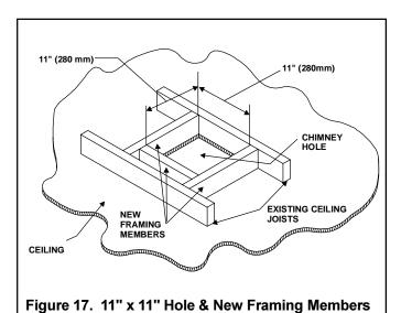
If the area above the ceiling is **NOT** an attic, position and secure the ceiling firestop on the ceiling side of the previously cut and framed hole.
